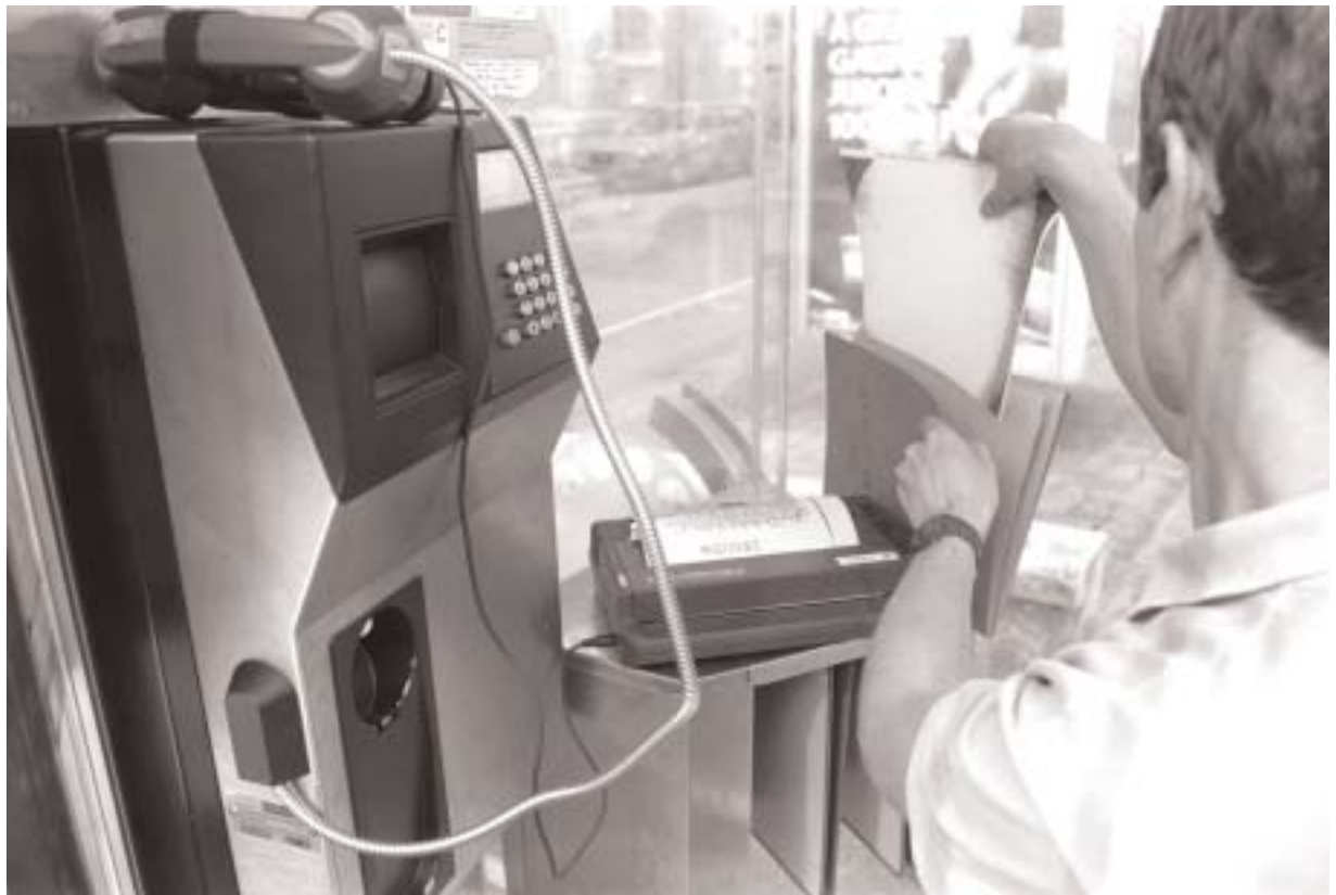
fig.3 :We used a telefax with acoustic modem that could be used in telephone booth or a car, and also when it was impossible to hook up a normal fax to telephone (which was a particular problem in Spain).When possible, however, we preferred to use a normal fax that was quicker and more reliable
